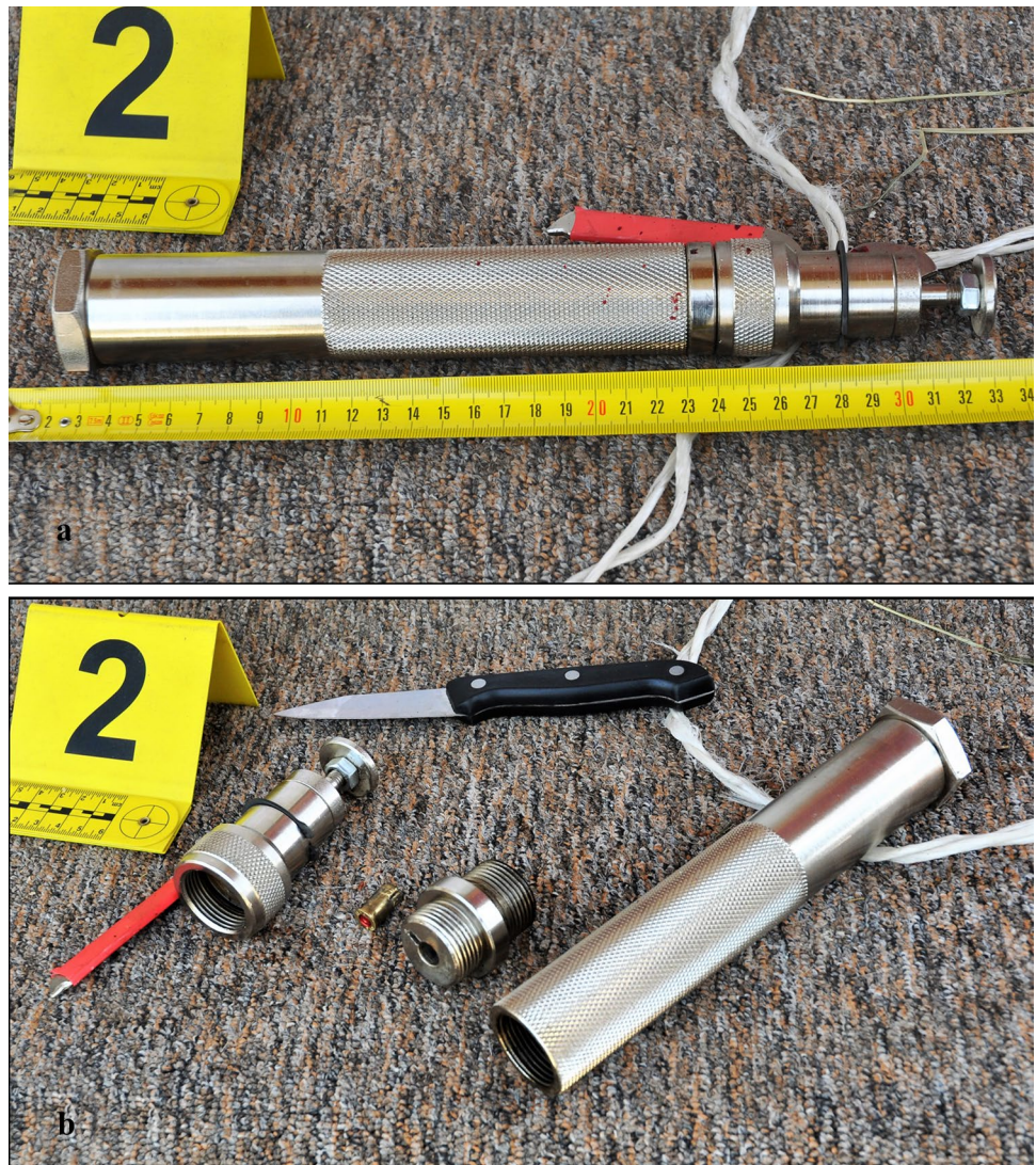
Fig. 2 The photographs were taken during police investigation. a Captive-bolt gun found on the scene. Note the blood traces on the gun. b Disassembled captive-bolt gun. Note the empty cartridge RWS 9×17
