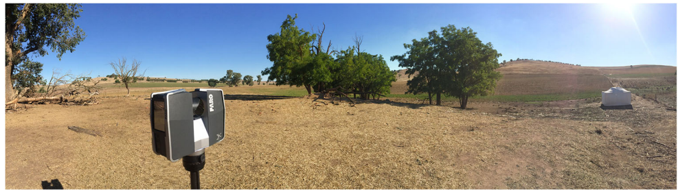
Fig. 4 FARO Focus s 70 terrestrial laser scanning (LiDAR) system utilized to image the siege area and develop 3D terrain models of the landscape
