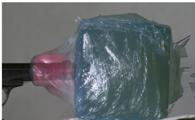
Fig. 2 Contact shot to model A. The plastic box ballooned in all directions. The original contact of the firearm with the target is deposited in the background
