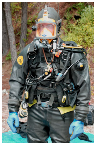
Fig. 2 Diver equipped with a full face mask and dry suit to dive in potentially contaminated water. A full face mask will also allow wireless underwater communication
