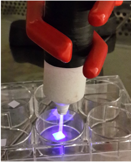
Fig. 1 Schematic of the instrument cold atmospheric plasma setup
