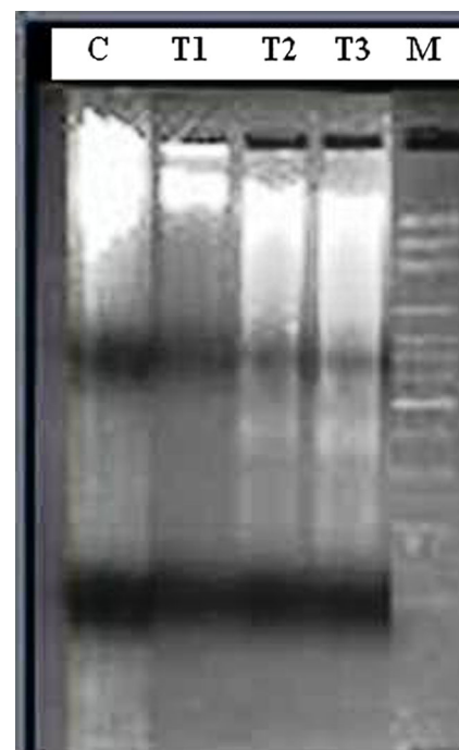
Fig. 4 DNA fragmentation pattern in HL-60 cells exposed to increasing concentration of ZnO NP for 24 h. C control, T1 0.01 mg/L, T2 0.025 mg/L, T3 0.05 mg/L of ZnO NP, and M 100-bp DNA marker
