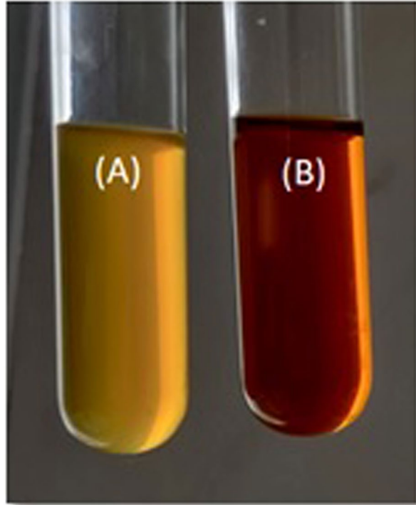
Fig. 3 Synthesis of AgNPs from Cassia tora seed extract A before synthesis of AgNPs, B After synthesis of AgNPs with Cassia tora seed extract. A Cassia tora seed extract + AgNO 3 , B AgNP from Cassia tora seed extract
