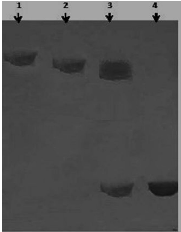
Fig. 4 The hydrolysed product of \alpha -amylase on TLC plate. Glucose as standard in lane 1 , maltose as standard in lane 2 , hydrolysed product of \alpha -amylase in lane 3 and unhydrolysed substrate (starch) in lane 4
