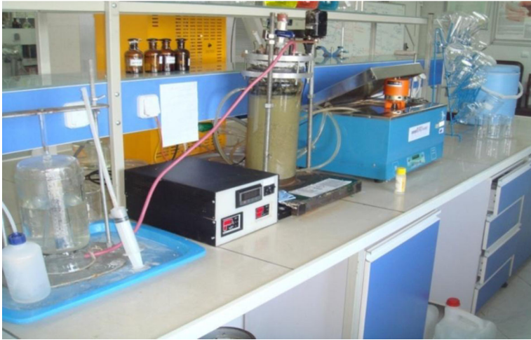
Fig. 1 The employed digester pilot of this study
