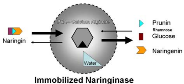
Fig. 1 Immobilization of naringinase in PVA–alginate for the hydrolysis of naringin
