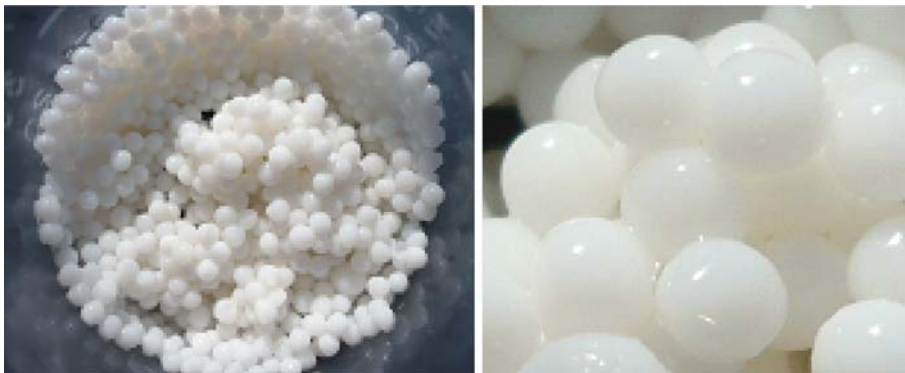
Fig. 3 Example of immobilized naringinase beads–PVA 10%–sodium alginate 1% cross-linking with boric acid 2%/calcium chloride 1% followed by sodium sulfate 10%. Size 2 mm
