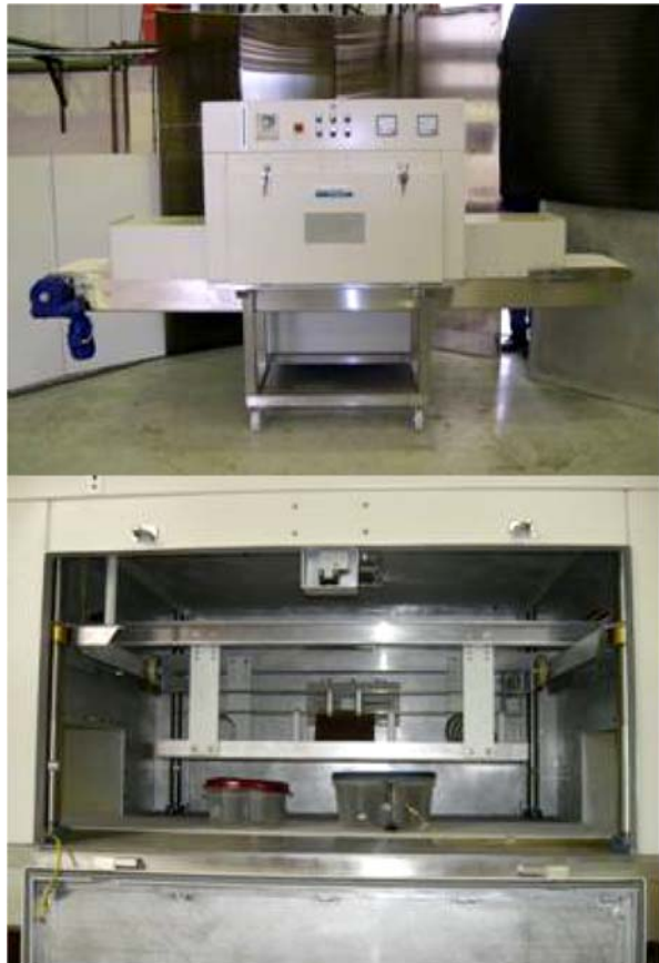
Fig. 1 Diagram of radio-frequency heating system
