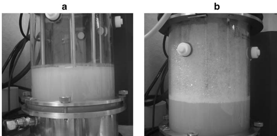
Fig. 2 Comparison between the rhamnolipid production with the conventional oxygenation and the one used in this work. a Nondispersive oxygenation. b Conventional oxygenation
