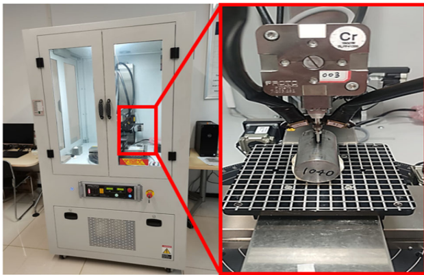
Fig. 5 Proto-LXRD 1200 machine set up for residual stress measurement
