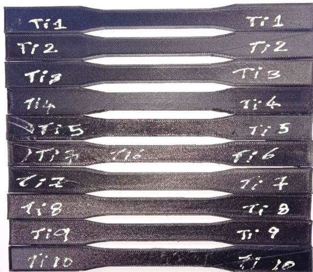
Fig. 3 3D printed tensile samples by C-Pla composite
