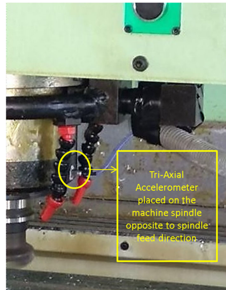
Fig. 1 Accelerometer placed on spindle for vibration measurement
