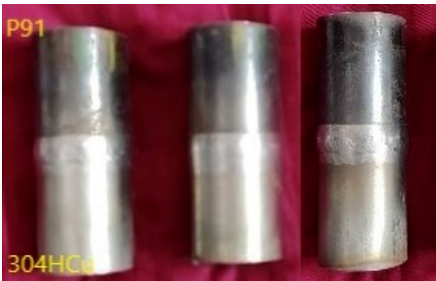
Fig. 4 Hot Wire TIG welded joints
