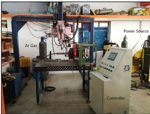
Fig. 3 Experimental Setup of HWGTAW
