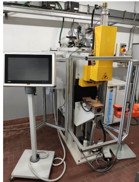
Fig. 2 RSW machine adopted during the experiments
