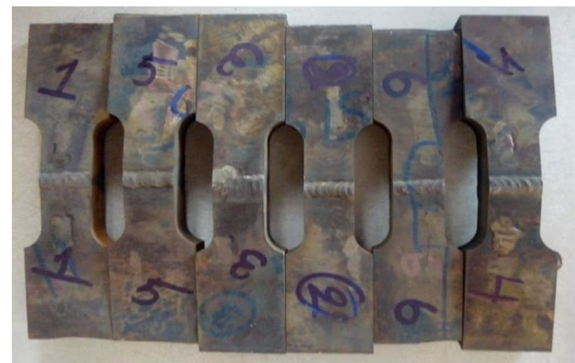
Fig. 3 Tensile test specimens as per ASTM D638
