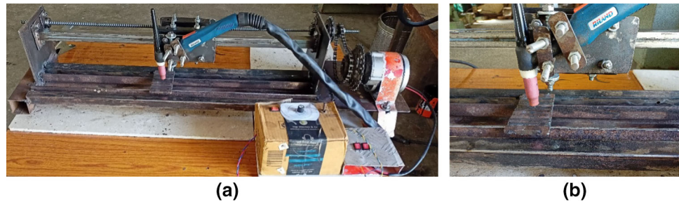
Fig. 1 Experimental setup for TIG welding a Chain sprocket and screw attachment for constant feed b vertical screw attachment used to control arc gap
