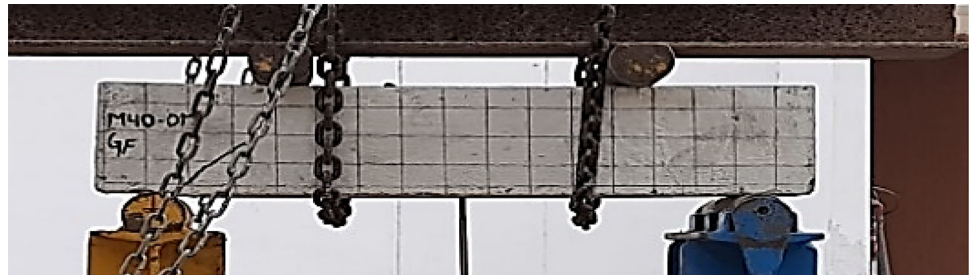
Fig. 3 Testing of concrete beams on a loading frame
