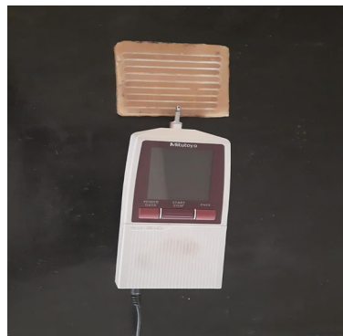
Fig. 4 Measurement of surface roughness using Form Talysurf
