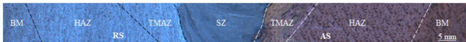
Fig. 12 Macrograph showing the cross section of the FSW sample for the confirmation test for the tensile strength experiment
