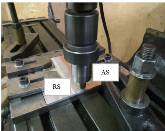
Fig. 2 FSW set up with welding strategy
