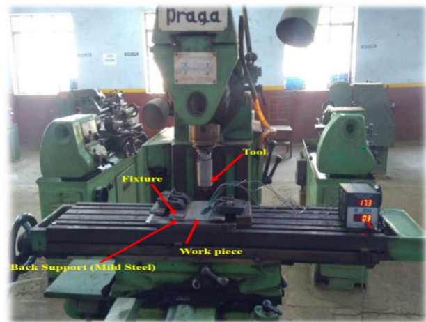
Fig. 1 Experimental setup of the FSW process
