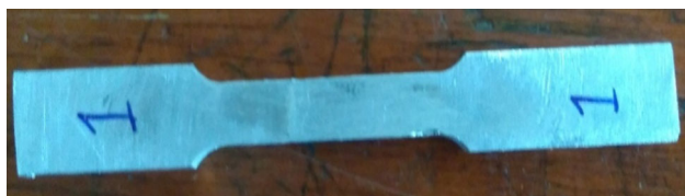
Fig. 4 Specimens for welded plates
