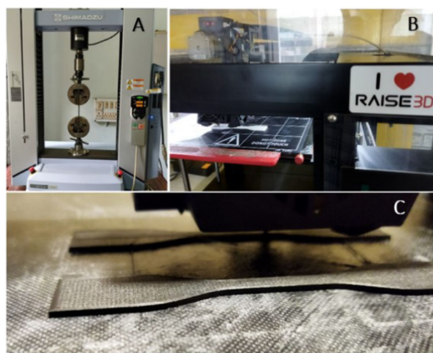
Fig. 4 a Ultimate tensile strength testing on Shimadzu AG-X plus, b FFF of PLA tensile samples, and c FFF of PLA-CF tensile samples
