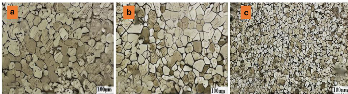
Fig. 8 Optical microscope images of a control sample b sample extruded at 350 °C c sample extruded at 500 °C
