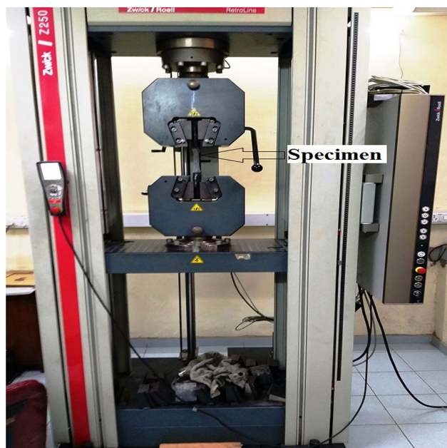
Fig. 9 Test specimen loaded UTM Machine
