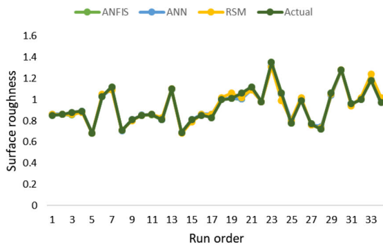
(a) Comparison of Actual (Ra) with predicted ANN, RSM and ANFIS predicted (Ra)
