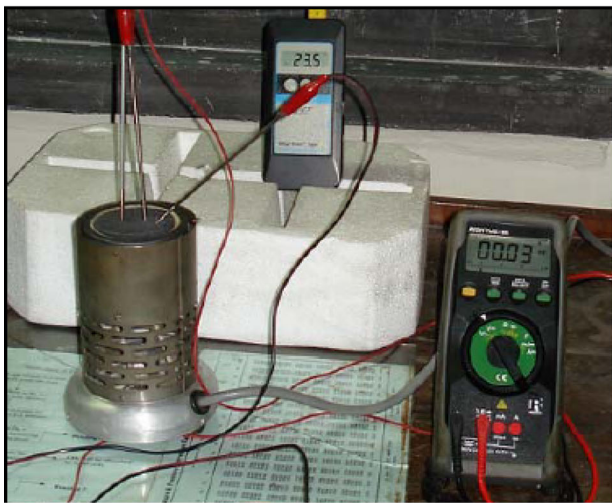
(b) Photographic view of the calibration set-up and temperature calibration curve for carbide and hardened medium carbon steel
