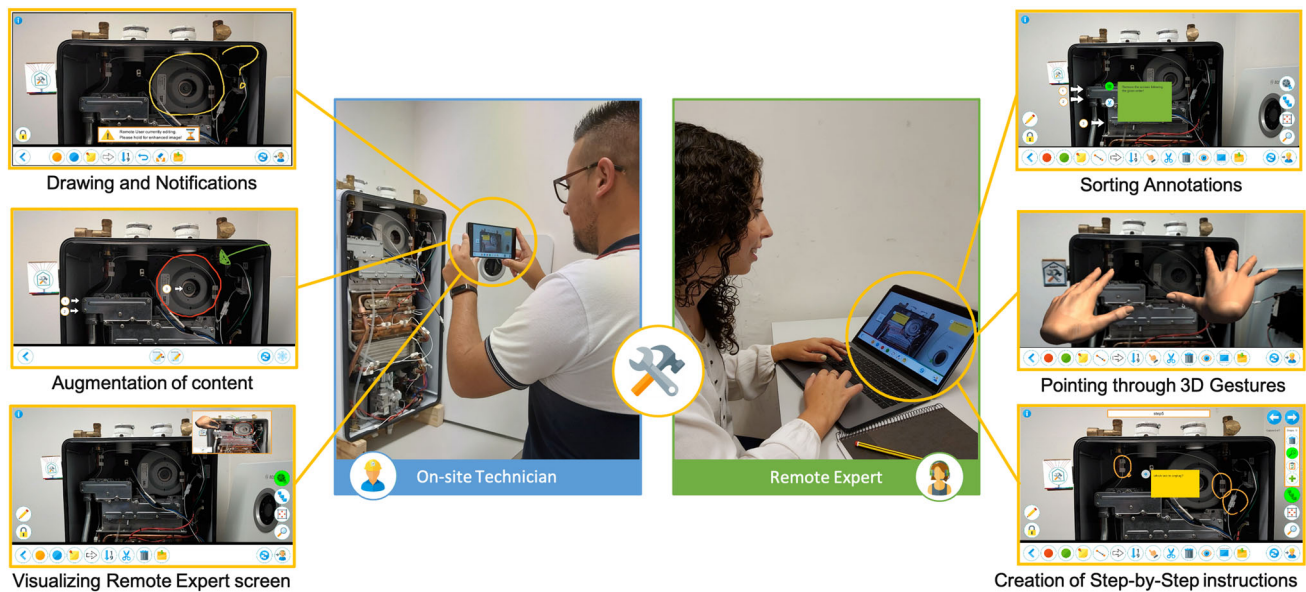
Fig. 5 Example of the prototype functions associated to the on-site technician (left: drawing and notifications; augmentation of content; visualizing remote expert screen) and the remote expert (right: sorting annotations; pointing through 3D gestures; creation of step by step instructions)
