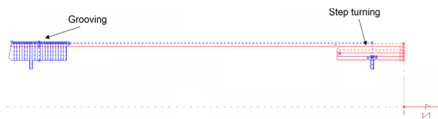
Fig. 15 Simulation of tool paths for the shaft
