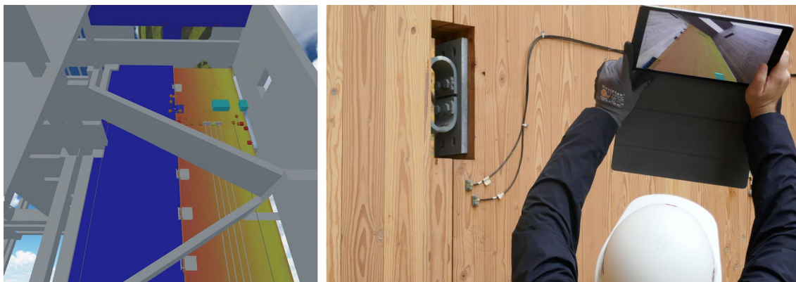
Fig. 4 Examples of representing the moisture content of a CLT wall with a heatmap in both the virtual reality and augmented reality setups. The locations of sensors are indicated with cyan-colored virtual objects rendered in each respective environment
