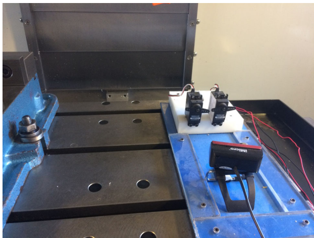
Fig. 7 Module of conventional servomotors on HAAS VF-2 table
