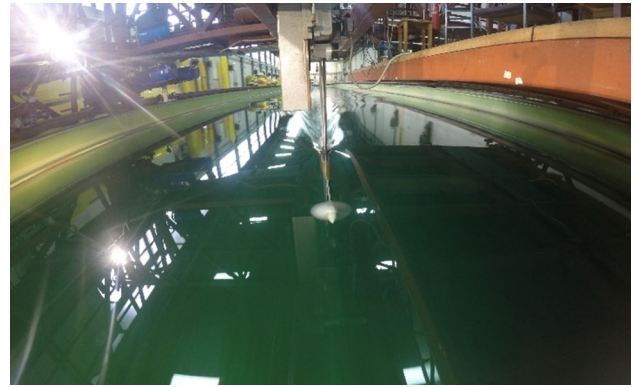
Fig. 9 The Towing Tank test using H29 propeller dynamometers
