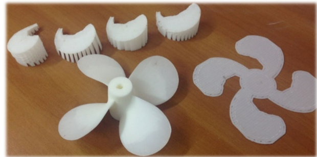
Fig. 3 The propeller printed in thermoplastic materials through the FDM process
