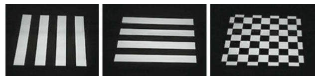
Fig. 5 Vertical and horizontal gray codes combined to produce a checkerboard pattern
