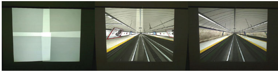
Fig. 1 Initial projector positions, geometrically corrected display and display corrected in geometry and colour
