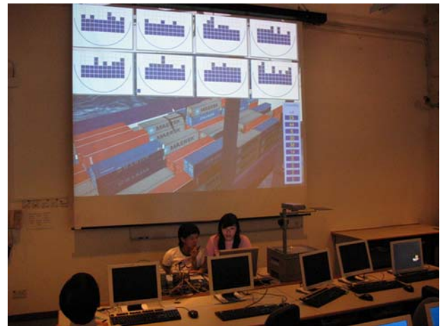
Fig. 8 Inside the virtual control room, the user interface displays the loading plan and container handling sequence that can be manipulated by the operators
