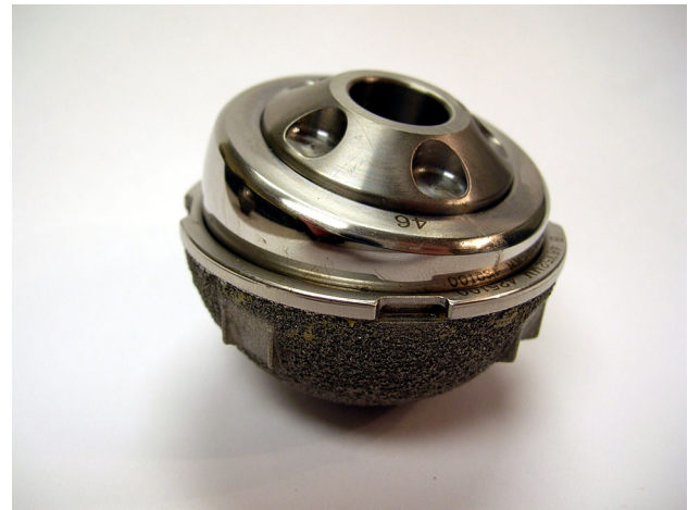
Fig. 2 The Magnum™ design (Biomet, Inc, Warsaw, IN, USA) was used in our center beginning in November 2004 through February 2010. It is a resurfacing style monoblock CoCr acetabular component coated with Ti-PPS and features a 3-mm fixed shell thickness, inner diameters up to 60 mm, and outer diameters up to 66 mm. It articulates with a modular CoCr head component that is effectively 6 mm smaller in diameter than the cup, which is mated with a titanium insert taper adapter.
