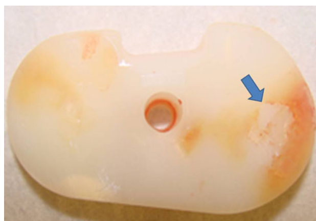
Fig. 2 Polyethylene insert from one of the retrieved cruciate-retaining TKA specimens with wear on the anterior half of the medial side of the insert indicating that posterior rollback is compromised in this case.
