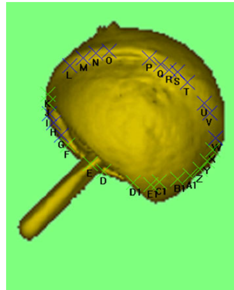
Fig. 1 An example of the 3-D CT image shows the cup face plane differentiated from the femoral head and the measurement points located around the rim of the cup.
