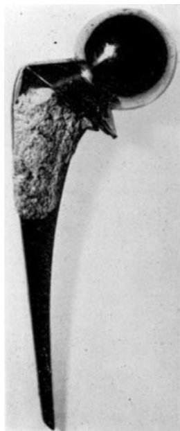
Fig. 15 An Austin Moore prosthesis inserted with cement showing the damage to the metal caused by the violence needed to extract it after one and a half years.
