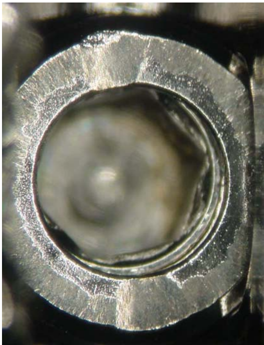
Fig. 6 This photograph shows average locking cap wear with rod dent.
