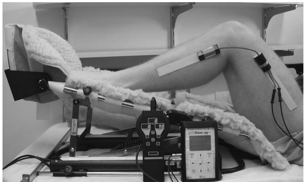
Fig. 1 A photograph shows a subject's leg with the electrogoniometer affixed along with the digital output unit and the CPM machine.
