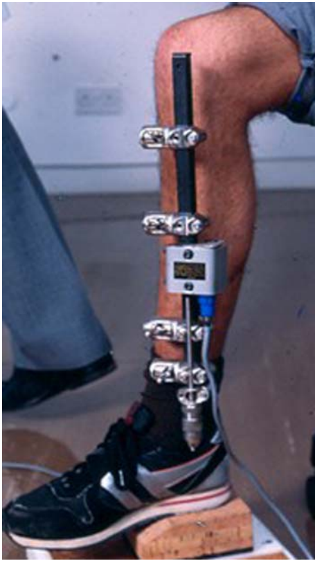
Fig. 4 Strain-gauged transducer device is attached to the fixator column to measure the loads acting on the fixation.
