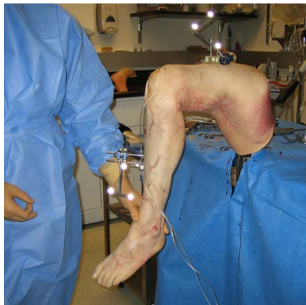
Fig. 1 The knee was mounted with the femoral axis parallel to the floor, and the navigation reference arrays were rigidly fixed with two pins per array.
