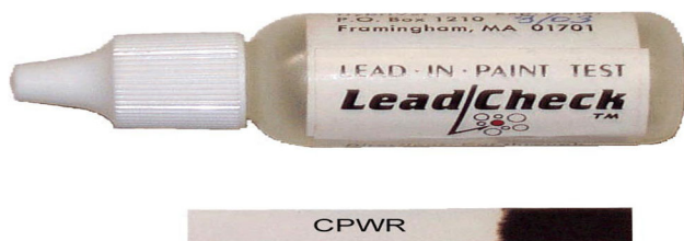
Fig. 7: Wet chemical field tests (like Lead Check®) 52
