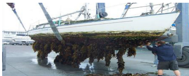
Fig. 6: Without antifouling paint coating 78
