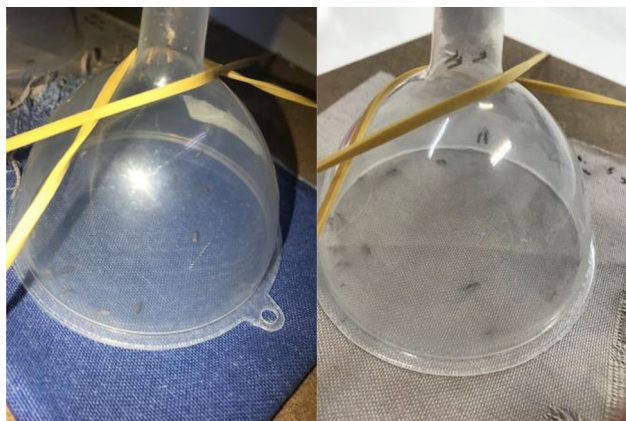
Fig. 2: Cone test for insect repellent effect
