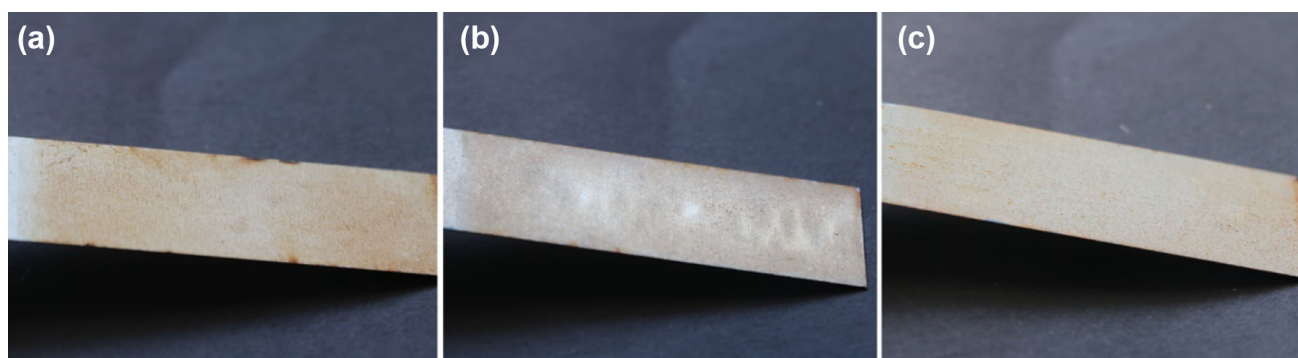
Fig. 15: Surface of corroded UV-curable EPD coatings with varying PIK contents: (a) WPA, (b) WPA-PIK5%, and (c) WPA-PIK15%
