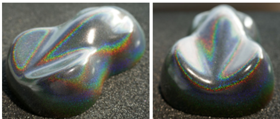
Fig. 1: Example of diffractive pigments used in coatings to produce a shifting multicolored effect on the object
