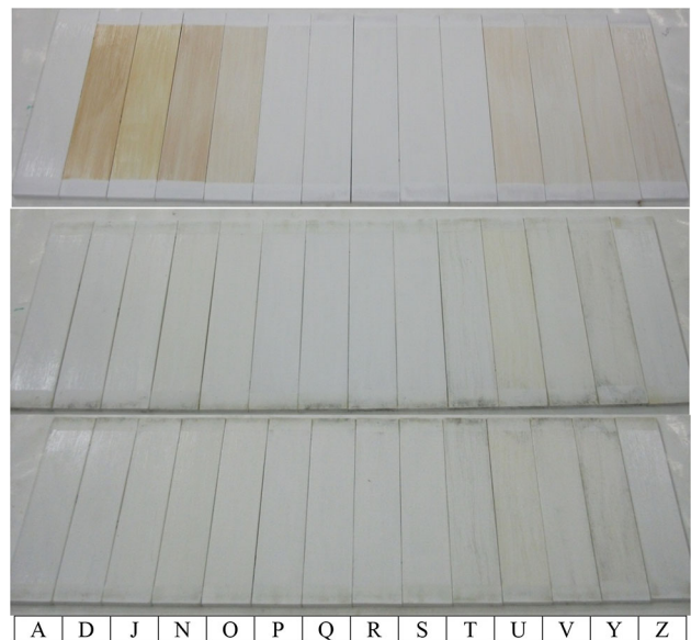
Fig. 9: Various styrene-acrylic coating samples applied over a white substrate after outdoor exposure. Original (top), at 38 days (middle) and 65 days (bottom)
