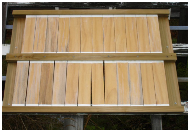
Fig. 8: Photograph showing various exterior exposure samples (as per Table 1) after 54 days outdoors. Samples A–F (bottom row) and samples G–M (top row), two specimens per sample are shown
