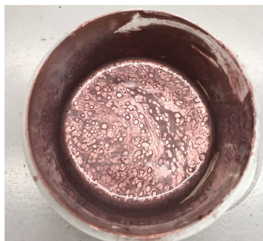
Fig. 7: Example of disadvantageous formation of air bubbles in the paste prepared by combination of binder and copper containing effect pigment
