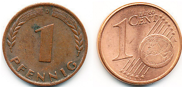
Fig. 5: Corrosion on copper coins as macroscopic model system for copper effect pigments, left: German Pfennig from 1967 and right: EuroCent from 2011
