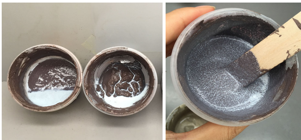
Fig. 6: Examples of failed binder/pigment recipes. Left with precipitation of pigments/right with oxidation of pigments
