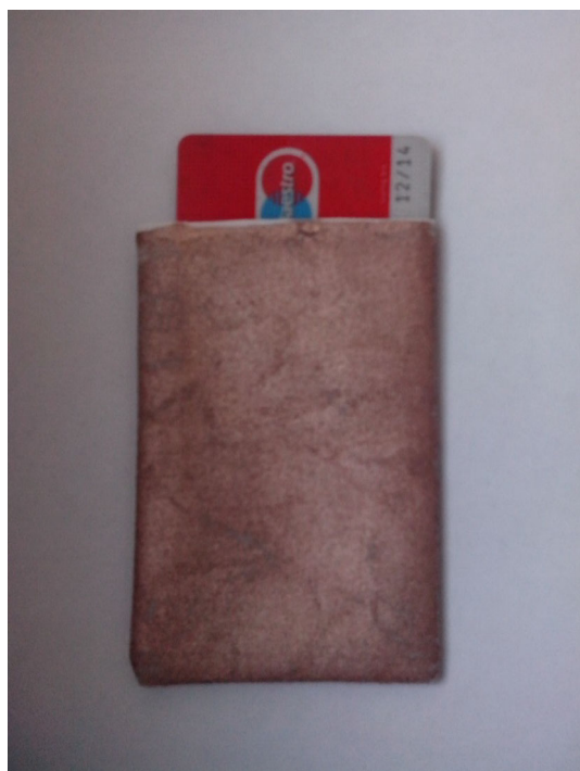
Fig. 13: Textile pocket with coating containing metallic effect pigment for EMI-shielding purposes
