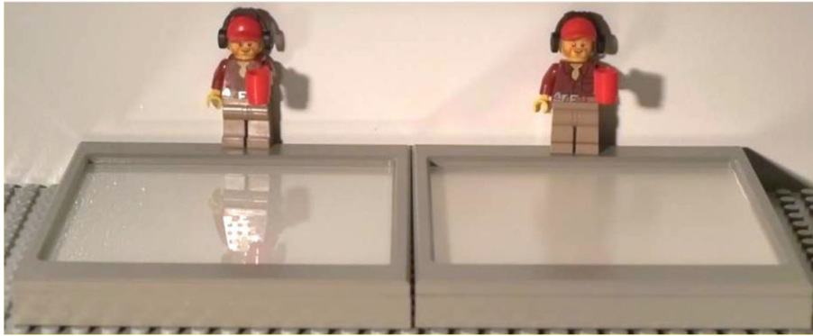
Fig. 2: Example picture of a white glossy (left) and a white semi-gloss (right) sample, developed as part of a gloss scale containing 40 artifacts. Both samples are illuminated with a uniform light source positioned above the samples. The left sample obviously possesses a higher reflectance; the lightness of the sample is higher and the image of the character in the sample surface can be better discerned
