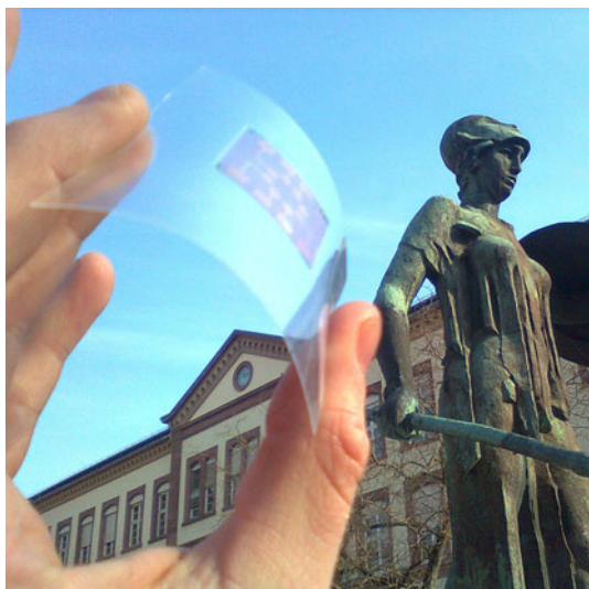
Fig. 1: Polymer-based solar cell, coated on a flexible PET substrate
